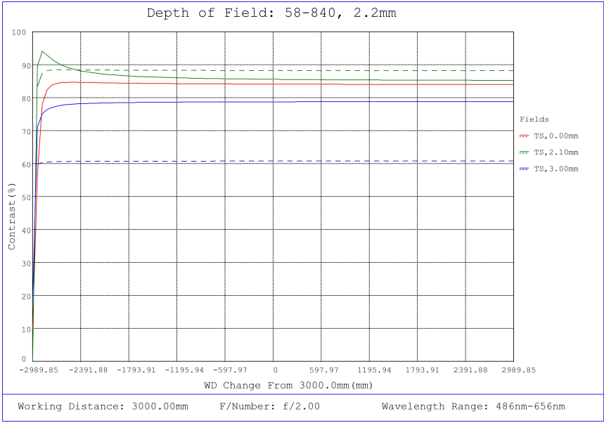
#58-840, f/2.0, Visible, 2.2mm HEO Series M12 Lens, Depth of Field Plot, 3000mm Working Distance, f2
