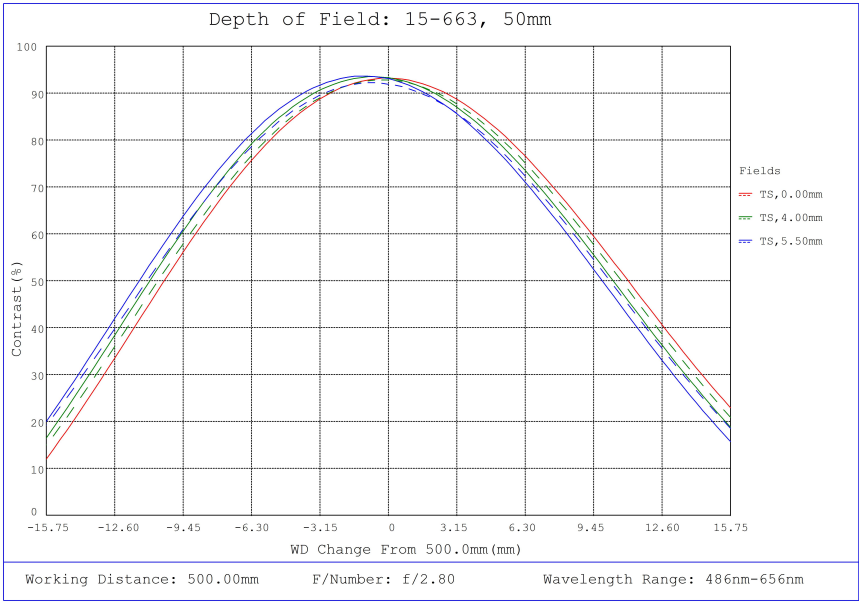
#15-663, 50mm, f/2.8 Sealed Cw Series Fixed Focal Length Lens, Depth of Field Plot, 500mm Working Distance, f2.8
