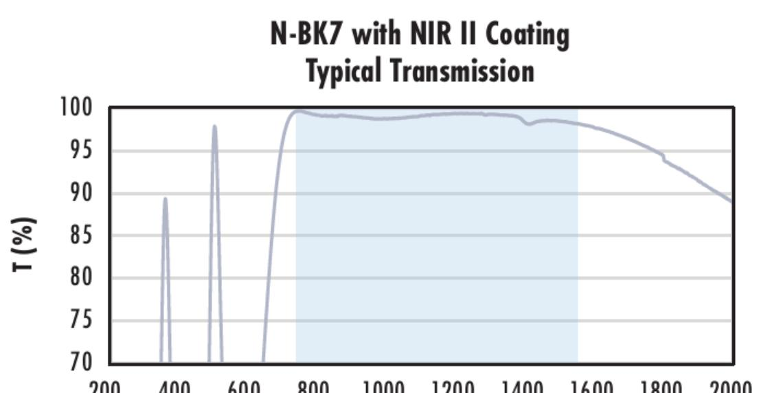
Typical transmission of a 3mm thick N-BK7 window with NIR II (750 - 1550nm) coating at 0° AOI.
