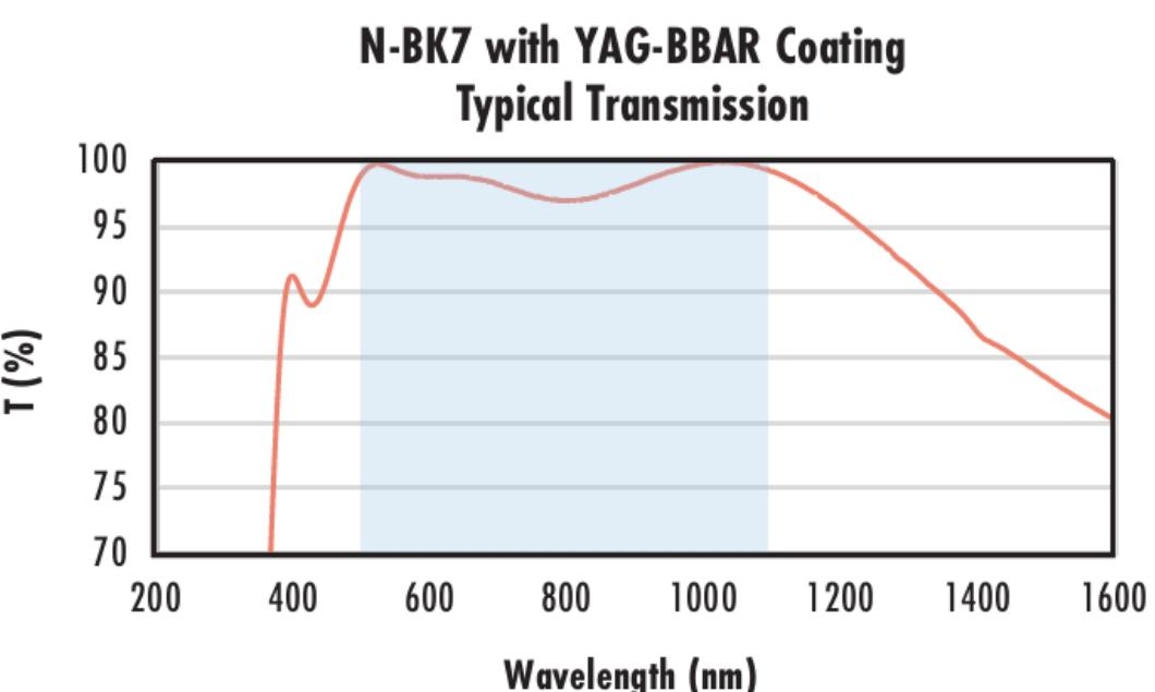
Typical transmission of a 3mm thick N-BK7 window with YAG-BBAR (500-1100nm) coating at 0° AOI.
