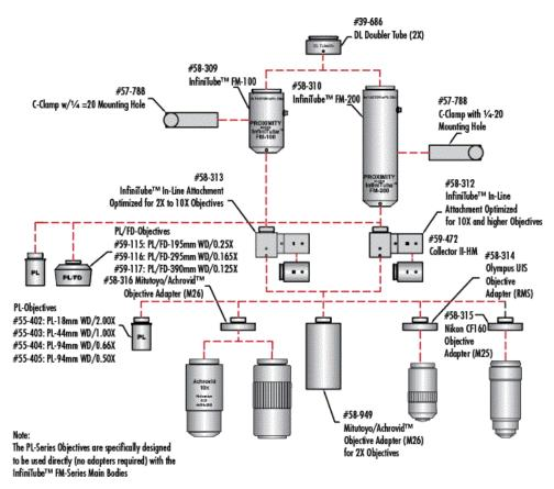
All PL-Series Objectives are amplified by 2X (InfiniTube FM-100) or 4X (InfiniTube™ FM-200) their engraved initial power ratings.
