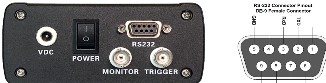
Figure 7 – Rear Panel with DB-9 Pinout (RS-232)
