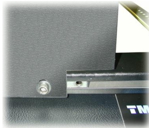
Figure 21, Keyboard shelf installation (View from below)
